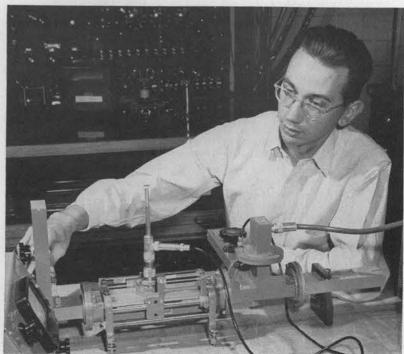
INTRICATE MECHANISMS are commonplace in the Electrical Standards Laboratory. Here, Merrill C. Jones checks VSWR measurements.
